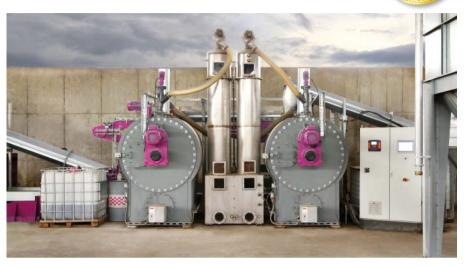
to already remove a large share of the nitrogen content in the biogas plant before its use in the biomass and to generate an ammonium sulphate solution, i.e. a known, permissible fertiliser, from it. In addition to the specific fertilisation effect, it is also very worthy of transport.
